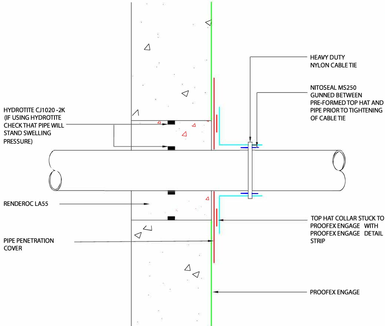
**PROOFEX ENGAGE SERVICE PIPE TOP HAT - POST INSTALLED PIPE**
