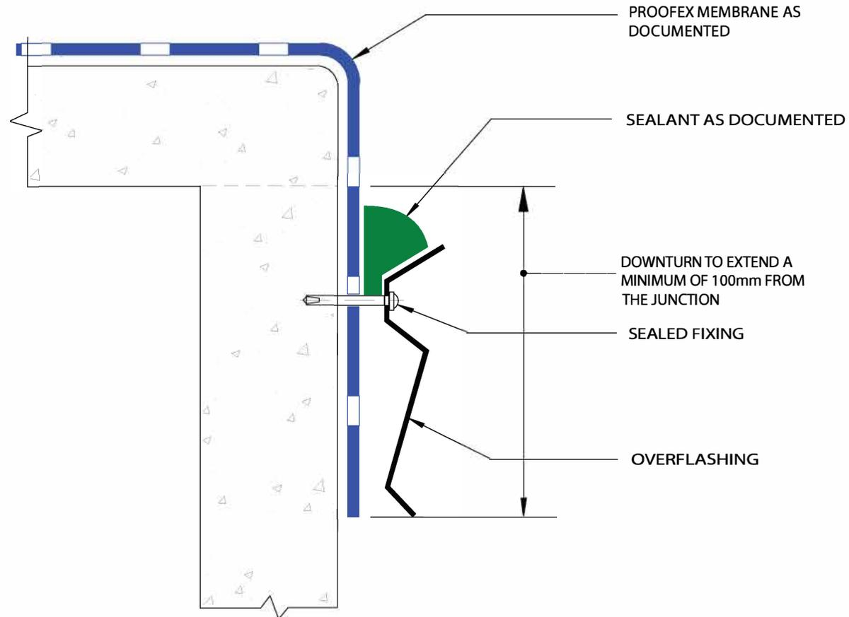
**PROOFEX - VERTICAL DOWNWARD TERMINATION WITH PRESSURE SEAL**
