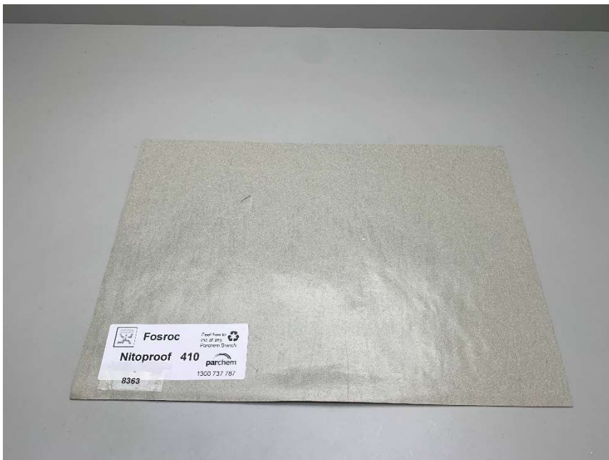
Figure 2 Underside of Nitoproof 410
