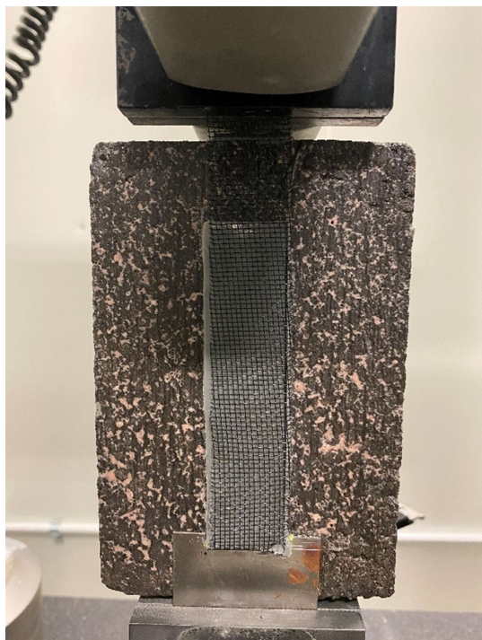
FIGURE 4 IMAGES OF TEST SAMPLE PERFORMING ADHESION-IN-PEEL
