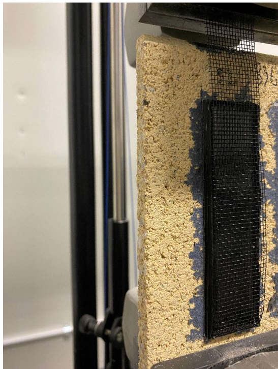
FIGURE 4 IMAGES OF TEST SAMPLE PERFORMING ADHESION-IN-PEEL
