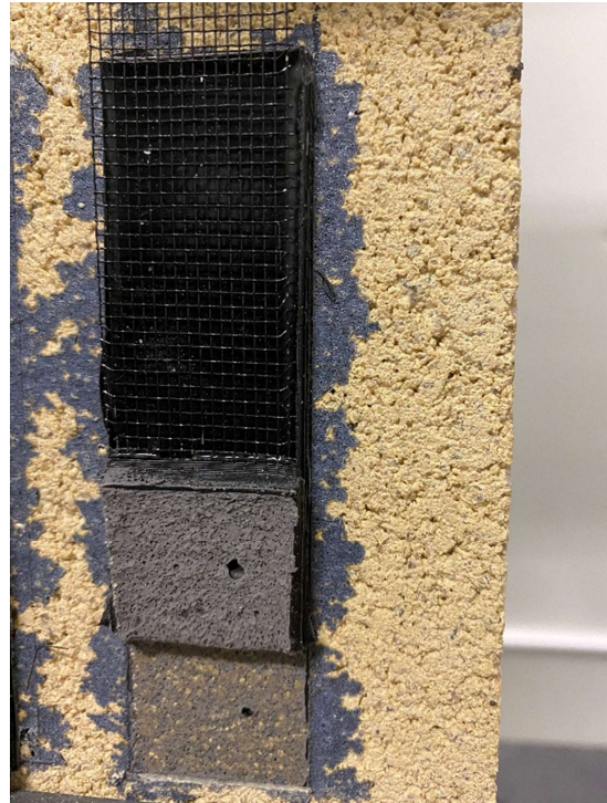
FIGURE 4 IMAGES OF TEST SAMPLE PERFORMING ADHESION-IN-PEEL
