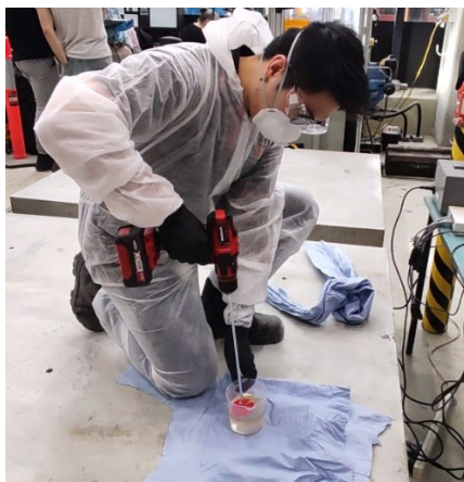
e) Mixing of Base and Hardener
